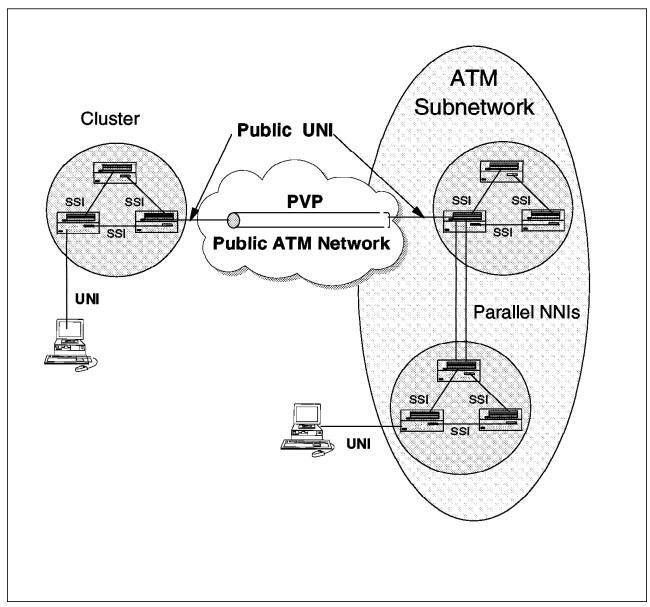
Figure 35. Complex ATM Network Using ATM 8285
